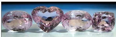
Fig. 2: Standard gemological tests, showed these pink gems to be spodumene, also known as kunzite.
